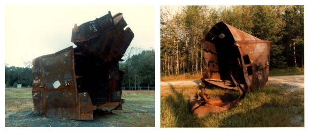
Structural failure from HE *detonation* Structural failure from propellant *burn*
